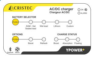
With the PUSH button of the BATTERY SELECTOR you can choose the battery technology and its associated charging curve. If you use the Bluetooth Cristec Connect application on your mobile phone or tablet and choose a different charging curve the CUSTOM led switches on.
