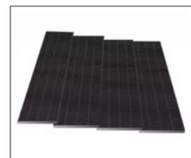
Shingled arrangement without gaps
